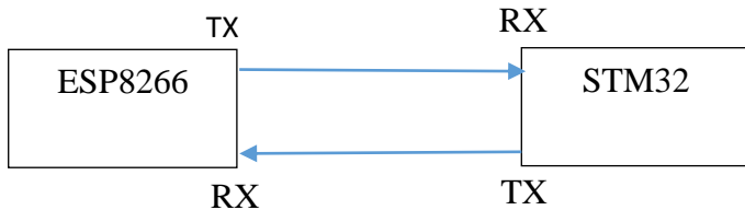
Fig. 31 – Interconnection between ESP8266 and STM32
